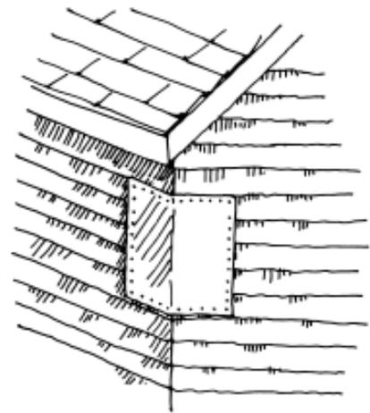
**Figure 3.** Raccoon access to rooftops can be eliminated by installing sheets of aluminum flashing, at least 3 feet square, around the corners of buildings.
