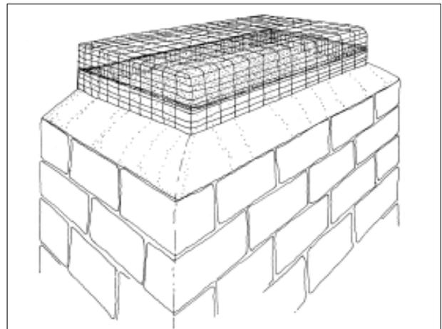
**Figure 5.** A commercially available chimney cap will prevent raccoons and other small animals from entering the chimney.
