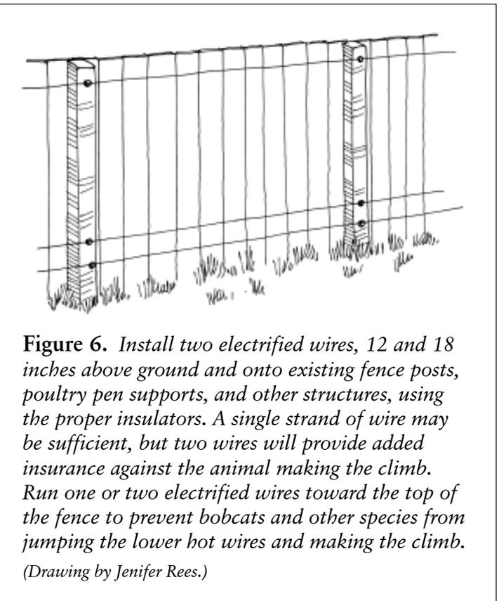
**Figure 6.** Install two electrified wires, 12 and 18 inches above ground and onto existing fence posts, poultry pen supports, and other structures, using the proper insulators. A single strand of wire may be sufficient, but two wires will provide added insurance against the animal making the climb. Run one or two electrified wires toward the top of the fence to prevent bobcats and other species from jumping the lower hot wires and making the climb. (Drawing by Jenifer Rees.)
