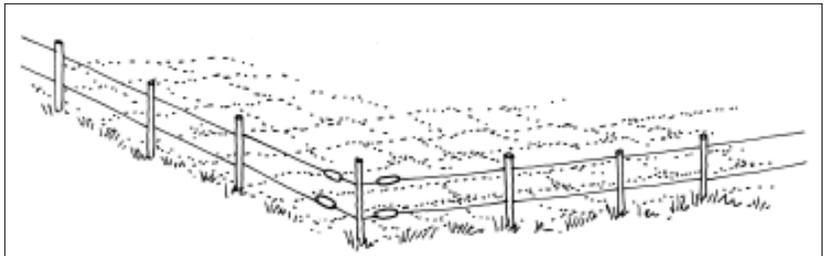
**Figure 8.** *Install two electrified wires, 6 and 12 inches above ground around field crops and other areas needing protection. The fence can be hooked up to a switch for discretionary use; when you want to work near it, turn the system off. Where the fence presents a safety problem, install signs, short pieces of white cloth, or other material on the wire for visibility.*
